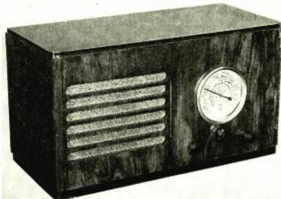
Fig. 11. Le Matériel Téléphonique (L. M. T. 43) five-tube (4 + 1) ac receiver with airplane type dial and station projection scales.
