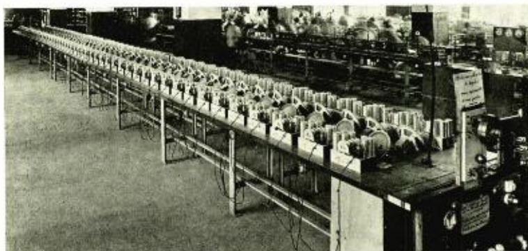
Fig. 17. Life test rack for 100 receivers, Boulogne factory.
