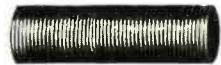
TYPE A RESISTOR—A column of resistor discs interleaved with silver discs upon which contact arm travels. Produces any resistance-rotation curve.
