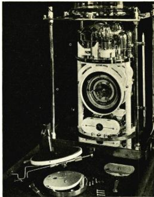
FIG. 3. CRYSTAL OSCILLATOR UNIT, SHOWING CRYSTAL ISOTHERMAL CHAMBER PARTIALLY OPENED.
