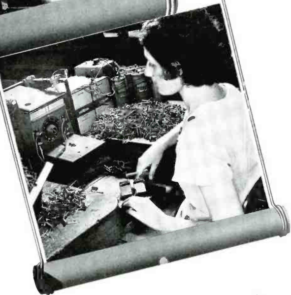
Top: An automatic machine of our own design that electrically tests and sorts Erie Resistors according to their tolerances.
