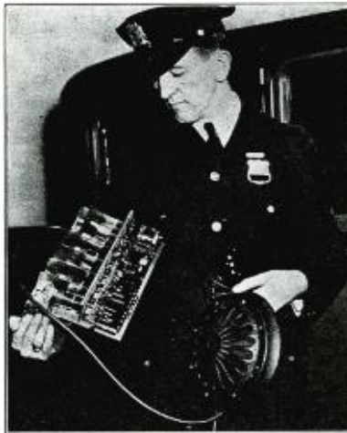
Courtesy Eveready Raytheon Company Automobile radio receiving sets used by the New York police department are simple in construction but sturdy and durable, built to withstand 24-hour service under all weather conditions.
