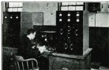
A 400-watt Western Electric transmitter in New York's police radio-telephone system. This one is located in Brooklyn; another identical one is located in the Bronx. The policeman, attached to the radio branch of the Telegraph Bureau, is broadcasting a message.
