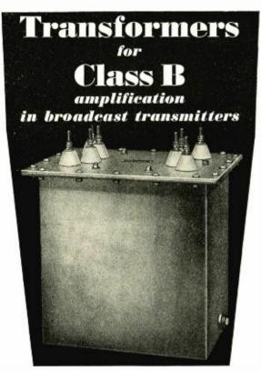
Output transformer for use between push-pull, class "B" stage using 204-type tubes and a class "C" amplifier. Operating level + 50d B; primary 1500 / 1500 ohms; secondary 4750 ohms; tested at 15,000 volts; oil insulated.
