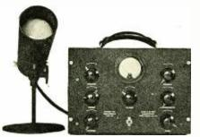
for use in connection with cathode ray tubes has recently been an-nounced. This amplifier consisting of three stages of resistance coupled amplification has a voltage gain of 500 and a useful range of from 10 to 500,000 cycles per second without distortion or appreciable phase bits shift.
