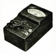
deep. Voltage ranges are 3, 30, 300 and 600. Resistance ranges are 0 to 1,000; 0 to 100,000 and 0 to 1 megohm. With minor wiring changes and the addition of IRC Precision Wire Wound Resistors, various d-c. current readings can be made. The basic meter used is an 0-1 millianmeter.
