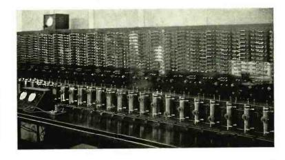
changes of as much as 70 per cent. in their resistance value. The new molded carbon type of control, under a test condition of 95 per cent relative humidity and 115°F, shows a change of less than 5 per cent over a period of 100 hours.
