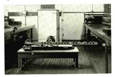
Fig. 1. In the foreground is the electrically driven "cycling" machine for making wear tests, both accelerated and extended. In the background is the huge humidity box wherein the volume controls are investigated in all conditions of humidity and temperature, while in operation and carrying current. The units on test are regularly checked for noise in special high-gain audio circuits with super-imposed r-f. currents.
