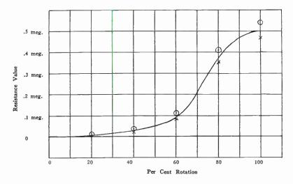
This curve is of a typical Stackpole molded carbon variable resistor, showing the changes due to (1) life test  $\{X\}$  and  $\{2\}$  humidity test  $\{\emptyset\}$ .
