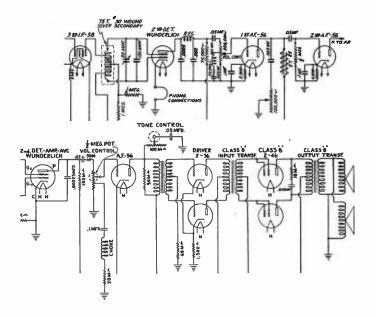
Fig. 4. These two circuits show the use of the "tapped" molded carbon volume control in the Clarion and Scott receivers to obtain automatic tone compensation. A tap on the regular audio volume control is connected with a series-resonant circuit to improve the low and high frequency response at low speaker levels to compensate for the response characteristic of the human ear. The circuits also show the application of these new control units for tone controls.
