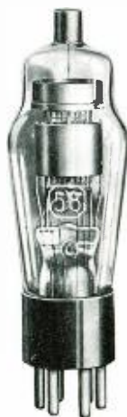
Type 58 tube containing SVEA METAL parts.
