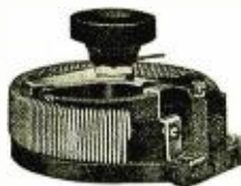
Fig. 1. An early type of variable resistor, used to control filament voltage. Note the lack of protection from dust, dirt and moisture.
