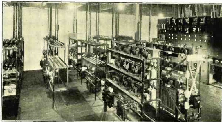
Fig. 1. Life testing racks.
