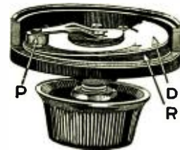
This shows the exclusive rocking disc construction of Centralab volume control. "R" is the resistance. Contact disc "D" has only a rocking action on the resistance. Pressure arm "D" together with shaft and bushing is fully insulated.
