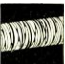
"Swimming" of wire after one coat of enamel is fused on
