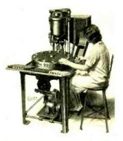
Machine indexes very smoothly and rapidly at fixed internals of time, regulated by three step pulley on motor. Base holding chuck rotates only when in filling position and automatic filling arrangement moves down to fill base. A uniform filling is assured by this method. A regulating cup Is filled with alcohol keeping free the filling device. Track arrangement lifts filled base, making removal of base easy.
