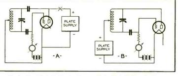
Fig. 4. Shunt-feed Hartley circuit. Series-feed Hartley circuit. Comparison of r-f. voltage with and without chokes.
