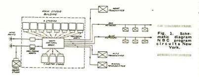
this system the switching is normally performed in the studios but is under the supervision of the control room supervisor who can detect and correct errors. The indicating lights on the master control desk show each operation involved in the switching of each studio and the supervisor can tell at a glance the status of any particular studio.
