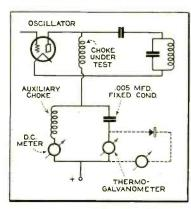
Fig. 3. One method of testing chokes.
