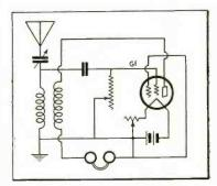
A one-tube receiver which requires no "B" battery.
