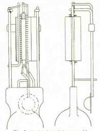
Fig. 2. Heater type tube assembly, for automatic manufacture.
