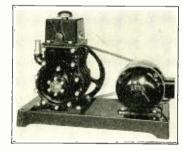
pump. At a speed of 425 r.p.m. it reaches a pressure of one micron in one fifth of the time required by the Cenco Megavace pump.
