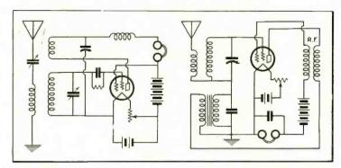
Fig. 3. Short-wave double-grid tube circuit.
