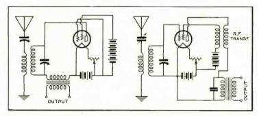
Fig. 5. This circuit shows the action of the tube as a rectifier. This circuit combined with that of Fig. 6, make the complete layout of Fig. 7.
