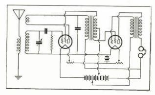
Fig. 15. Twotube receiver the equivalent of three stages of audio amplification. A four-element tube (tetrode)¹ will often give good signals with no plate battery. In portable receivers the plate battery takes space and adds weight, so the set is improved if no plate battery is necessary. A simple circuit for this purpose is shown in Fig. 14. A separate antenna coil will make it more selective.
