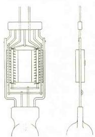
Fig. 1. Early 5-voit heater tube assembly,
