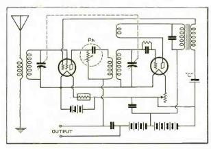
Fig. 8. Radio receiver using a double grid tube and a regenerative detector - the equivalent of a three- or fourtube receiver.
