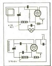
Fig. 9. A form of super-regenerative receiver.
