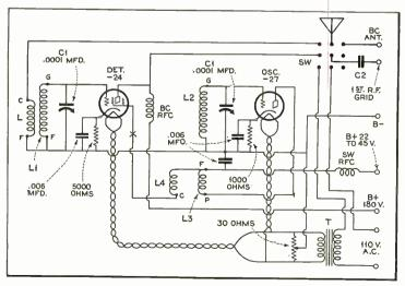
Fig. 1. Circuits of Tanner converter.
