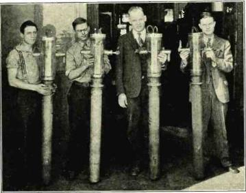
High Power (100 kw.) vacuum tubes, by General Electric Co.
