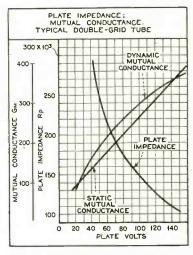
Fig. 11. Plate impedance and mutual conductance of typical double-grid tube.
