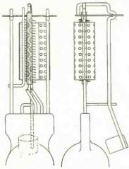
Fig. 8. Construction of perfected quick-heater audion.
