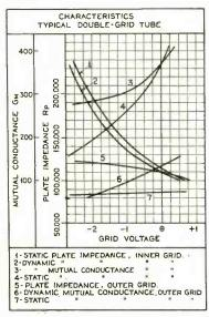
Fig. 12. Characteristics of double-grid tube
