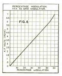
from the data in Fig. 5 and gives the peak values of a-c. to be applied across the resistance to obtain the desired modulation percentages.
