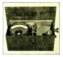
Fig 2. Mutual inductor attenuator without cover.
