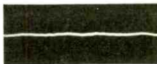
Oscillogram showing noiseless performance of Bradleyunit Resistors.
