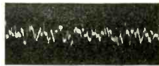
Oscillogram showing noisy performance of other types of resistors.
