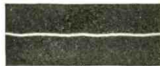
Oscillogram showing noiseless performance of Bradleyunit Resistors.
