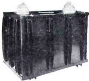
Fixed condenser type 2244 for use in electric (induction) furnaces—capacity (air) 4450 mmf. In castor oil 20900 mmf. May be operated on 140 amperes at 300 KC continuously without overheating.
