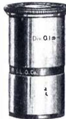
Fig. 42. An ocular micrometer containing a permanent calibrated circular glass. (Courtesy, Bausch & Lomb)
