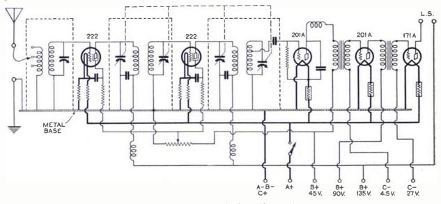
A typical band selector circuit, with tuned plate and grid circuits, which provides a rectangular resonance curve.
