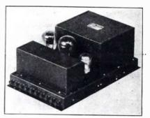
Webster power amplifier single 250 tube. amplifier using a
