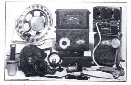
The complete transmitting and receiving apparatus for airplane communication. At left the fairlead, heimet with headset, flame-proof key, and at right, the microphone.
