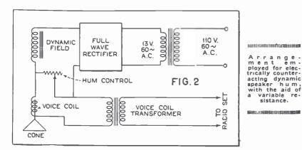
but also introduces an impedance of the movable coil at higher frequencies.
