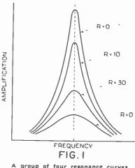
A group of four resonance curves of tuned radio-frequency circuits.
