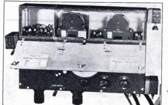
The five-tube receiver has wavelength ranges of 50 to 150 meters and 580 to 1100 meters. Notice the special suspension mounting clamps, which facilitate mounting. The weight is approximately 11 pounds.
