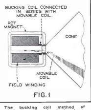
The bucking coil method of eliminating dynamic speaker hum.
