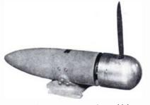
The wind-driven generator, which supplies all the necessary current for operating the transmitter and receiver.
