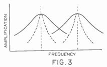
Illustrating the effect of regeneration on a tuned R.F. circuit. Selectivity is increased, as indicated by the dotted curves.
