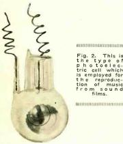
Fig. 2. This is the type of photoelec-tric cell which tric cell which is employed for the reproduc-tion of music from sound films.
