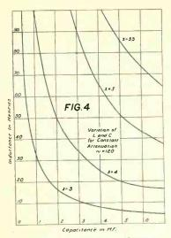
Curves showing the proper induct-ance and capacitance to give vari-ous values of attenuation.
