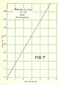
Curve showing the relation be-tween loss in TU and attenuation.
