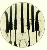
Fig. 3. Nickel supports (marked by arrows) pressed in the glass stem of a tube. There is an absence of gas bubbles, causing cracked stems. (Transmitted light; specimen immersed in monochlor benzol. Mag. 5.)
