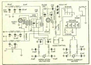
The schematic diagram of the specially designed standard signal generator.
