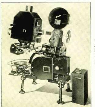
Fig. 5. A West-ern Electric projector for sound pictures, on which is used a Simplex head. A Pow-ers or Motio-graph head may also be em-ployed.
