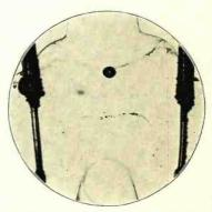
Fig. 7. The continuous row of bubbles on the left seal wire caused a leak in this stem. The right seal wire was satisfactory. (Transmitted and reflected light: specimen immersed in monochlor benzol. Mag. 9.)
