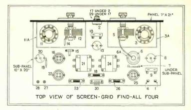
Detailed constructional layout for the receiver described. Note that the R.F. and detector circuits are enclosed in aluminum shields.
