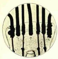
Fig. 4. The nickel supports marked by arrows show correct amount of gas. That one marked by an X was untreated before using and contains too much gas. (Transmitted light; specimen immersed in monochlor benzol. Mag. 5.)
