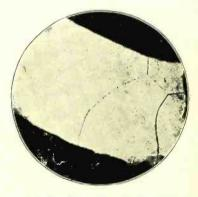
Fig. 2. The piece of tungsten here shown was burned in an oxidlzing atmosphere and shows oxide contamination along the grain boundaries. Mag. 50.
