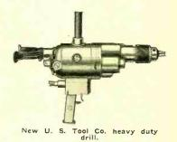
running in grease. Double silk insulated, enameled, armature wire. One-piece, aluminum body frame and commutator head. Quick make, quick break, two-pole trigger switch. Three-jaw screw back chuck for straight shank drill bits, etc. This new model weighs only 27 pounds, and sells at \$75.
