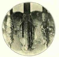
Fig. 5. Same as Fig. 3. Note the cracks in the glass stem due to the too complete union between the glass and nickel. (Transmitted and reflected light; specimen in air. Mag. 11.)
