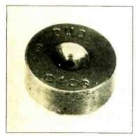
(Photo. courtesy of Detroit Wire Die Co.) A diamond die for drawing No. 14 to No. 50 gauge wires.
