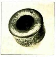
Chilled cast iron die for drawing No. 3 to No. 14 gauge wires.
