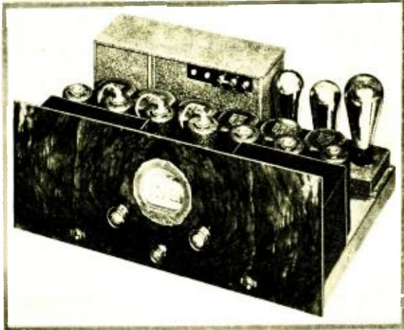
The Tyrman Imperial "80", a receiver of the superheterodyne variety, employing A.C. screen-grid tubes in the intermediate amplifier and a 350 power tube in the output. The power supply equipment is housed in the metal case at the rear of the chassis.
