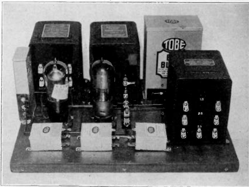
Above: Sub-base layout of the apparatus forming a convenient power plant for A.C. operated sets. Below: Layouts of the fixed and variable resistors, and the voltmeter on the panel.
