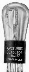
The new Arcturus 127 A.C. replacement tube which has a 2.5 volt filament. It is claimed that this tube reaches full emission more rapidly than the standard—27 type tube.
