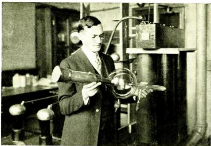
H. F. Tanis, Jr., holding one of the new Coolidge cathode ray tubes
