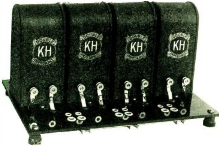
The completed tuned double impedance A. F. amplifier. The last unit is an output filter
