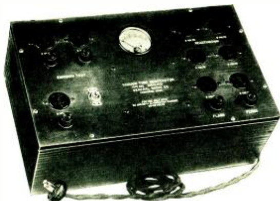
A vacuum tube reactivator which operates from a 110 volt 60-cycle line. Sockets are provided for testing, flashing and cooking. The correct voltages are maintained automatically.
