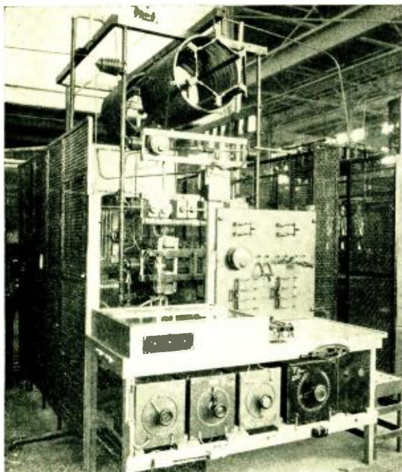
A front view of one of the test sets for checking up on completed water-cooled Pilotrons and Kenotrons. One tube can be seen mounted in the test rack.
