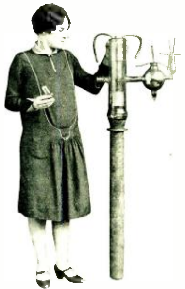
A 100 KW water cooled transmitting tube, contrasted with a 199 type receiving tube.
