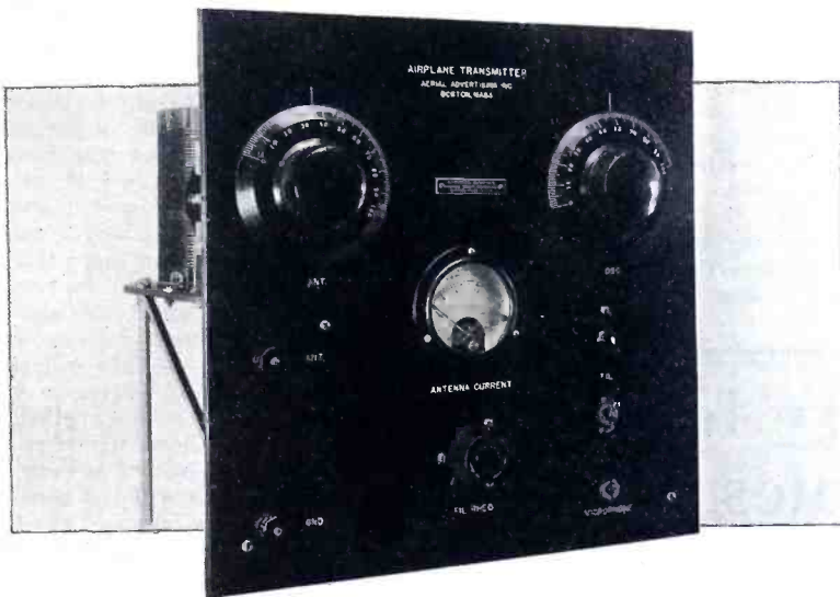
A radio telephone transmitter for use in talking between airplane and earth—designed by the National Company, Cambridge, Mass.
