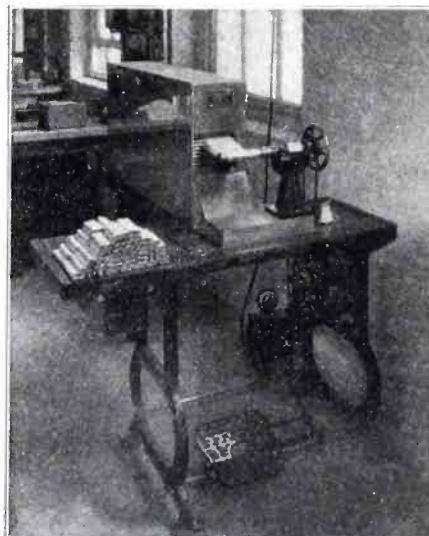
Fig. 1. A special winding machine was designed to keep all foreign matter from the paper and foil
