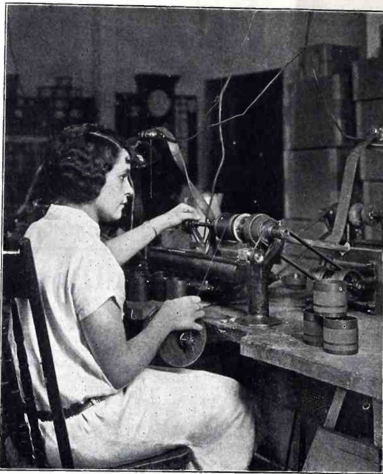
Fig. 1. The machinery and method employed for winding plain coils or tubing
