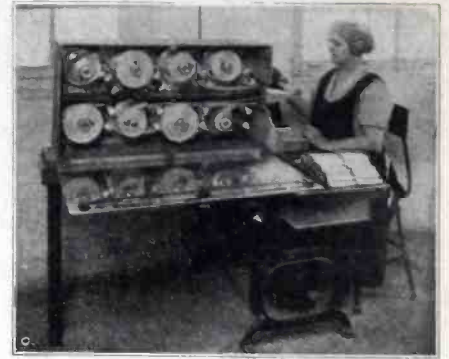
Fig. 2. A side-view of the winding machine, exposing the reels of alternate paper and foil
