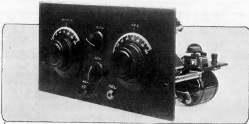
Fig. 1. The front panel, tho only 14-ins. long, carries the double-rotor coupler and two S. L. F. condensers
