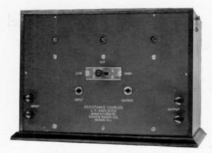
A neat and efficient instrument is the Daven resistance coupled amplifier. Another type, of less expensive construction, is now available, equipped for three or for four stages of amplification. Since the increase in volume per stage is directly dependent upon the amplification factor of the tubes, UV-201-A's must be used for best results.
