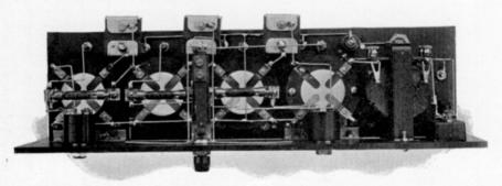
Fig. 4. This view shows the method used to mount the Daven coupling resistances on the Paragon sockets. Be sure to have the jack switch upside down as it appears here.
