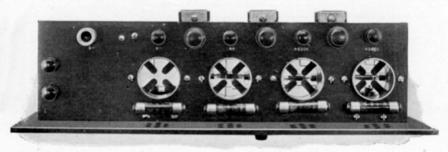
Fig. 6. Locking down on the tube panel you can see the Variohm control knobs and the Amperite filament current regulators.
