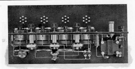
Fig. 1. Note the way in which the Micadons are supported on the Variohms, and the method of mounting the upper and lower parts of the Kantblo.
