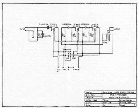
Schematic wiring diagram and circuit constants for the Daven amplifier.
