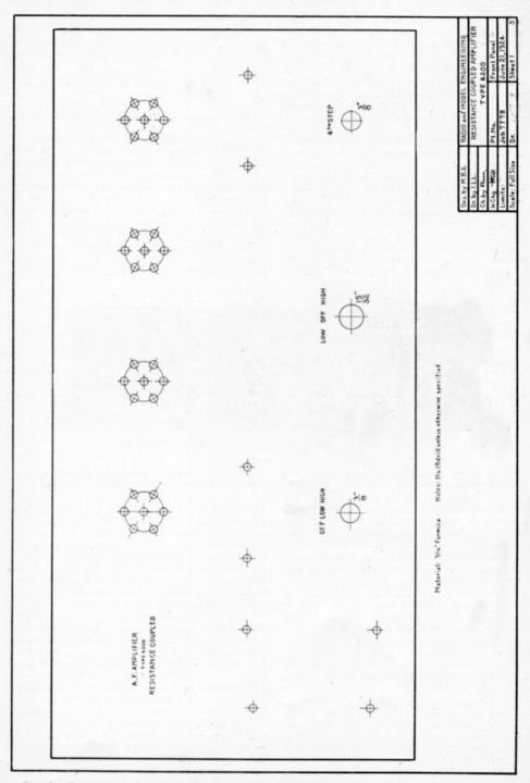
Fig. 3. The front panel at one-half scale. Make all holes with a No. 18 drill except where other sizes are specified.
