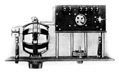
Fig. 2. Only two wires running to the tube panel are required. The rest of the connections are supplied by the panel supports
