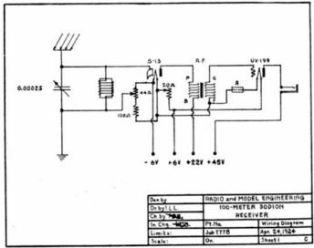
Fig. 2. Wiring diagram of the Sodion set for 100-meter reception
