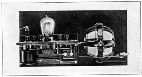
Fig. 1. The fixed crystal, mounted at the left of the tube, can be seen, as well as the supporting arrangement for the socket
