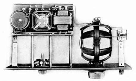
Fig. 6. Looking underneath at the works of the set. You can see the R. F. transformer, socket, and A. F. transformer
