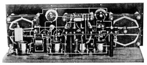
Rear view of the outfit removed from the cabinet. Note the construction of the D coil variable transformers
