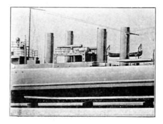
Fig. 9. Here the bridge shows more plainly. The tall ventilator is made by mounting an ordinary short ventilator on a wooden dowel. The life boat and the torpedo tubes are illustrated also. Port holes can be turned out of brass tubing. or they can be purchased either plain or fitted with glass
