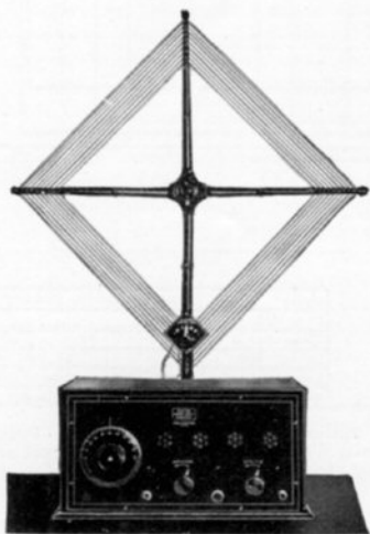
The loop is carried on a bracket secured to the rear of the cabinet. Thus the loop can be rotated without interfering with the operator
