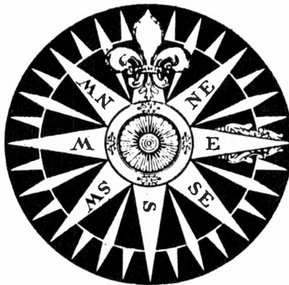
FIG. 6—USE A PHOTOCOPI of this artwork for the top of the compass, and glue it in place on top of the case.
