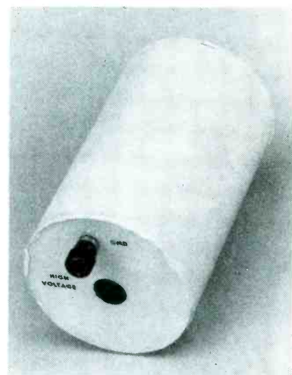
FIG. 2—THE "CABINET" for L1 can be fashioned from a cardboard tube. The end caps can be made of plexiglass.
