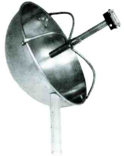
FIG. 8—THE PROTOTYPE BIG EAR-TYPE microphone. The tubing containing the microphone and the amplifier is positioned for optimum sound pickup.
