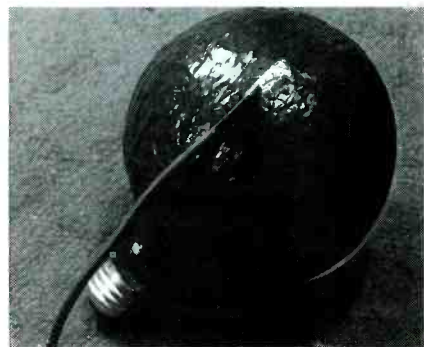
When applying the second layer of tape, leave a small area of aluminum exposed, and connect a wire to the foil.
