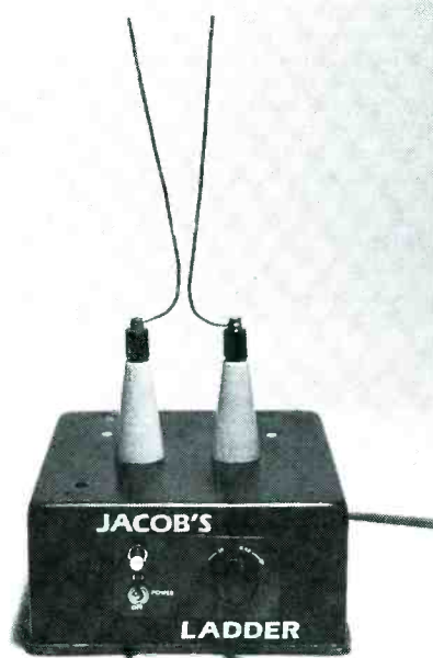
FIG. 3—ANOTHER JACOB'S LADDER. The transformer used in this model permitted the use of a low-profile baking-pan chassis.
