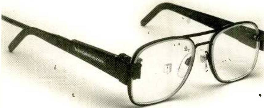
The original version of the prototype eyeglasses head mounted display that has been developed by MicroOptical Corp. The electronic components including the AMLCD are located in the frame.
