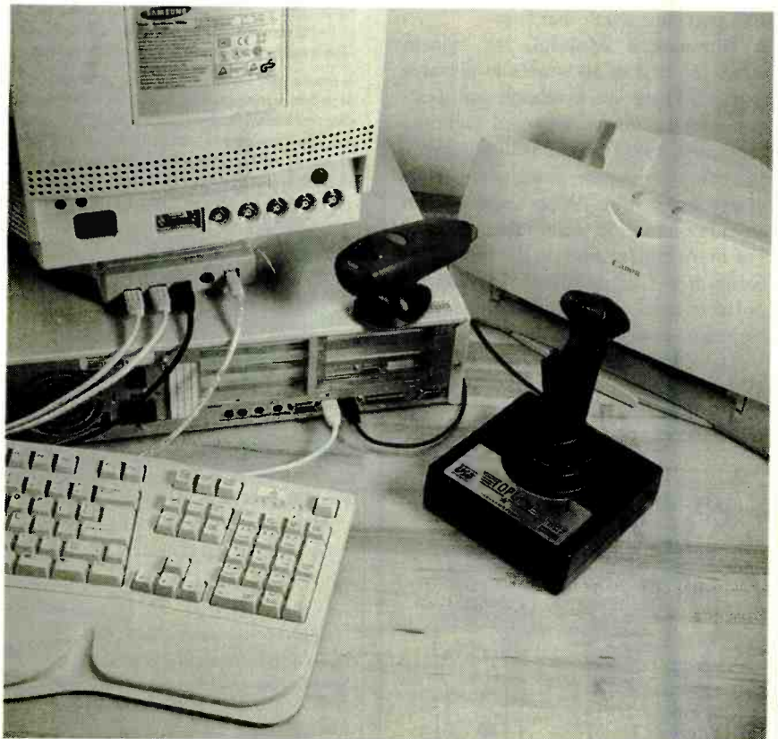
WITH USB (AND AN APPROPRIATE NUMBER OF USB HUBS), you can daisy chain up to 127 peripherals to your computer, including printers, joysticks, digital cameras, keyboards, and mice.
