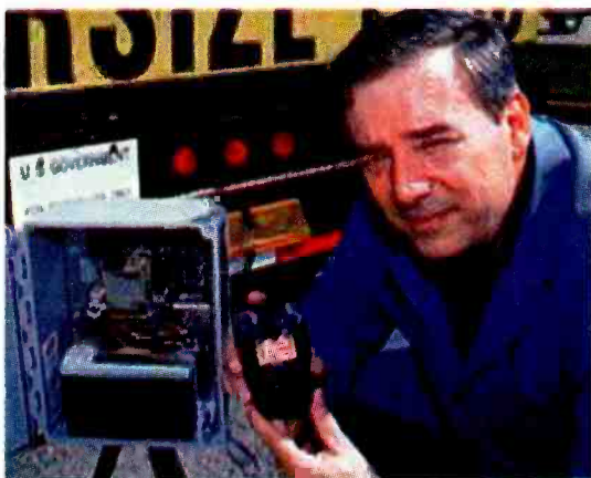
RESEARCHER GENE GRENEKER is refining and field testing a device he developed called SWS, a microwave-based communications system that warns motorists of hazardous driving conditions ahead.
