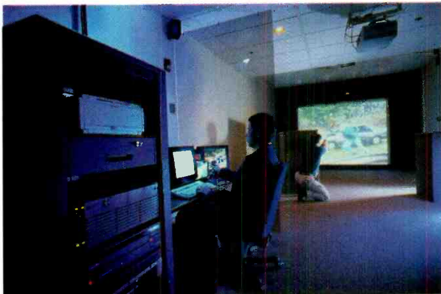
THE PRISim SIMULATOR includes a 10 × 10 ft projection screen and sophisticated computer control to simulate real police “use-of-force” situations.
