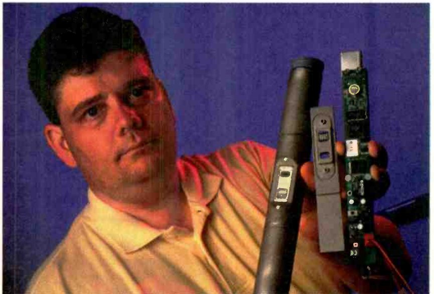
RESEARCHER JEFF MOORE HOLDS environmental monitors that contain integrated optic interferometric sensors developed at Georgia Tech.
