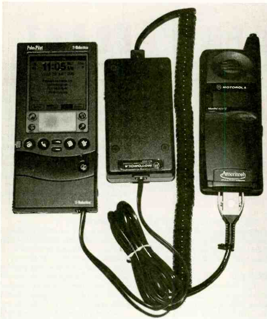
FIG. 1— WIRELESS E-MAIL IS POSSIBLE USING A PILOT, a modem, a cell phone, and a black-box adapter. The modem clips on the Pilot, and the adapter connects between the cell phone and the modem.
