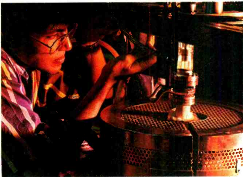
DR. PROBAL BANNERJEE, post-doctoral fellow at Auburn University, adjusts the operation of a viscometer, during measurements on a cast-iron alloy.
