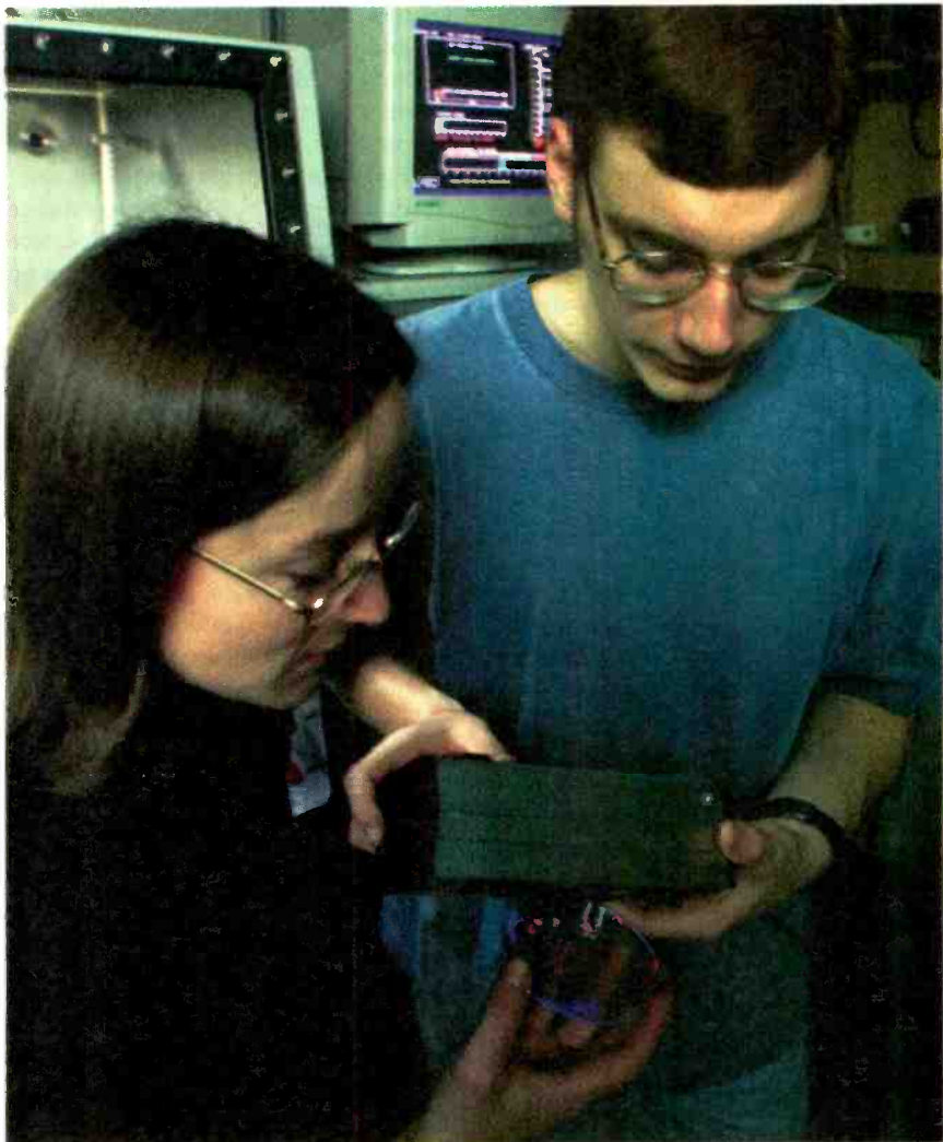
PERDUE STUDENT MATTHEW ALLEN shines ultraviolet light on a dish containing small gray structures made of porous silicon, causing the structures to emit a bright orange light. Principal researcher Jillian Buriak is shown at the left. (Purdue News Service Photo by David Umberger)
