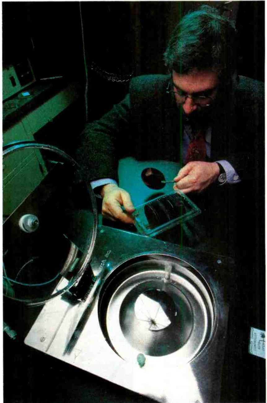
RENSSELAER RESEARCHER JOEL PLAWSKY is shown here removing an aerogel-covered wafer from a climate-controlled spin coater.
