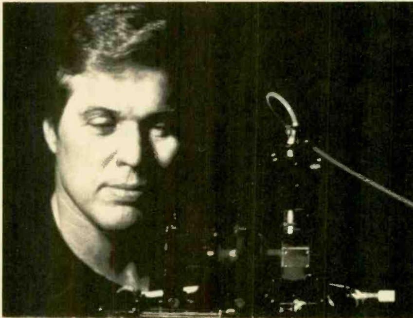
Project manager Paul Gourley examines a semiconductor diode laser's beam used to excite the VSCEL biocavity laser. The VSCEL releases an invisible infrared beam which carries information about cells to a detector.
