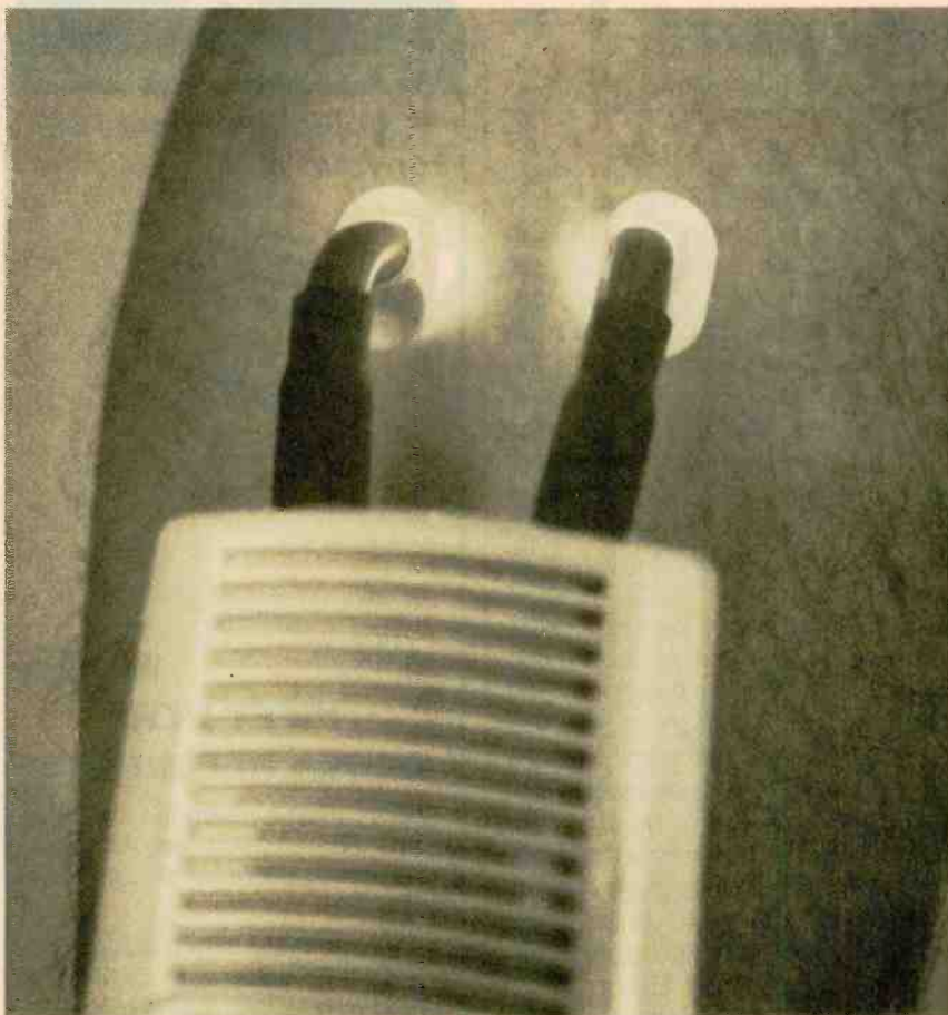
The Venoscope uses a dual light source to transilluminate the veins from two sides of the device, making them easier to find.
