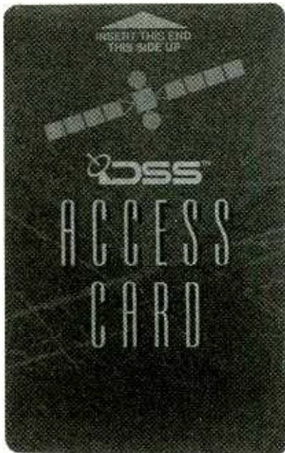
THE SMART CARD or access card for the DSS integrated receiver/descrambler (IRD) has drawn the attention of hackers.
