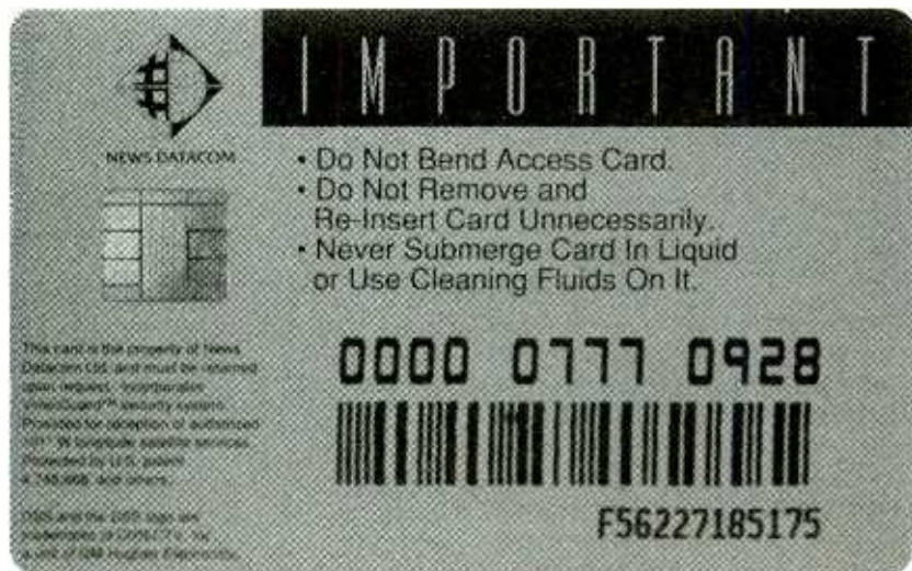
THE BOTTOM OF THE SMART CARD shows its contact points. Note News Datacom's patent statement that hackers credit with helping them.
