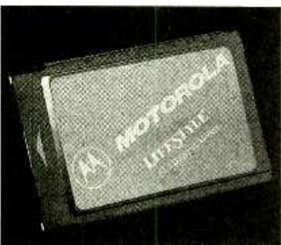
FIG. 8—THE MOTOROLA LIFESTYLE PC-Card data/fax modem can send and receive data at 14.4 kilobits per second.
