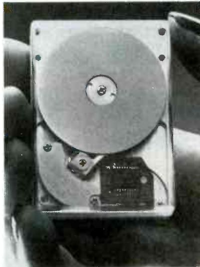
HEWLETT-PACKARD'S 1.3-INCH DRIVE shown here actual size.
