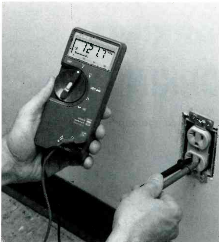
FIG. 1—A BASIC DMM, like the Fluke Model 70, is an indispensable tool for LAN troubleshooting.
