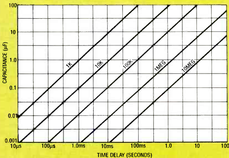
FIG. 3—COMBINATIONS OF RESISTANCE AND CAPACITANCE yield a range of time delays. The trigger pulse width must be less than the timing period.
