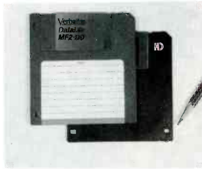
FIG.1—A SECOND HOLE INDICATES that a disk is high-density.
