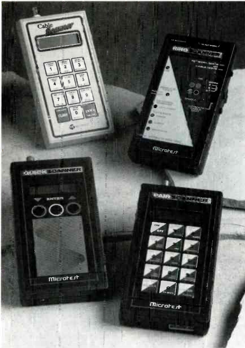
FIG. 2—MICROTEST'S HANDHELD LAN TESTERS combine most-needed features in easy-to-use, hand-held packages. Clockwise from upper left are the Cable Scanner, the Ring Scanner, the Pair Scanner, and the Quick Scanner.
