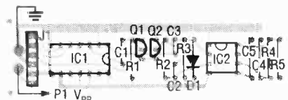
FIG. 14—EPROM PC BOARD. Mount all parts except J1 on the component side of the board; mount J1 on the foil side.
