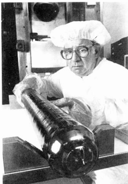
WESTINGHOUSE TECHNICIAN Don Nebel holds a single-crystal boule of silicon, believed to be the purist and largest ever produced.
