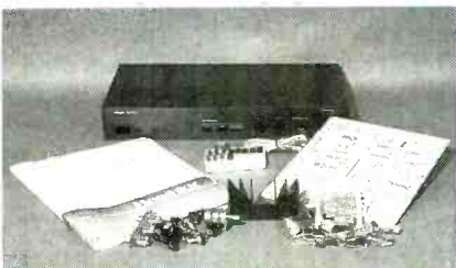
MOST OF THE ASSEMBLY work is done on a large PC board.
