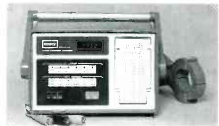
FIG. 5—THE DRANETZ SERIES 901 POWER HARMONIC ANALYZER, similar to a BMI 2400. In one printout for an instant in time, the device records line voltage, the current used, total power, power factor, harmonic power, fundamental power, and a breakdown of the power in the individual harmonic frequencies above the fundamental (in other words, its spectral content).
