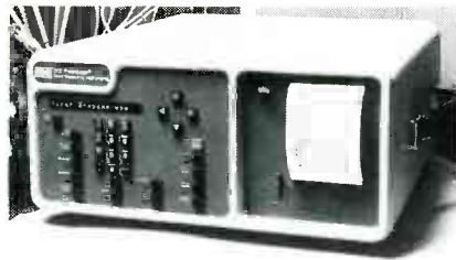
FIG. 3—THE BMI 2400 POWERSCOPE power-transient measurement and recording system for single-phase DC, or single- or 3-phase AC. The instrument monitors sags, surges, impulses, waveshape faults, line-frequency variations, and high-frequency noise for single-phase AC or DC, has a built-in RS-232 bus to be used with an external processor to analyze total harmonic distortion and frequency spectral content, and has a full range of available accessories, including temperature and humidity sensors.
