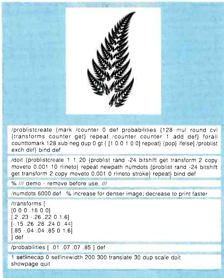
FIG. 5—A FRACTAL FERN DONE IN POSTSCRIPT. Note that only 28 data values are needed to completely define this image. But what's really astounding is that you don't really "draw" this fern—instead, you simply let it out!
