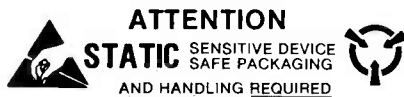
FIG. 5—ALWAYS USE PACKAGING labels like this one to indicate ESD-sensitive parts, and that proper handling of the parts is required.
