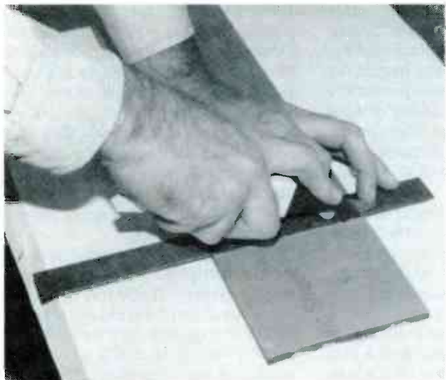
FIG. 5—DON'T TRY TO CUT THE PLEXIGLAS with a saw. Instead, use a straightedge to guide the scoring tool.
