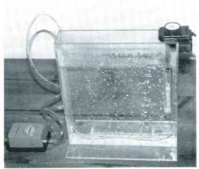
FIG. 10—HANG THE HEATER from the side of the tank, connect the air bubbler, and check for an even bubble distribution.
