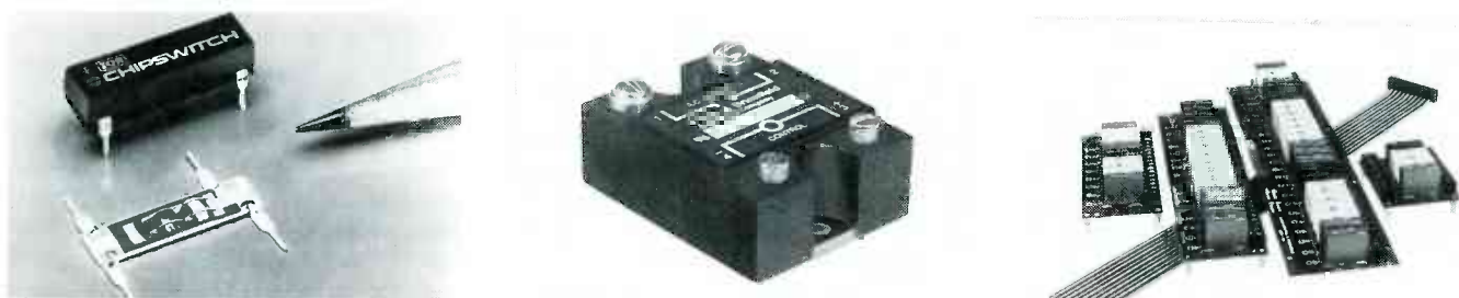
FIG. 7—THE THREE most common solid-state relay styles are the (a) IC DIP, (b) power, and (c) I/O module varieties.
