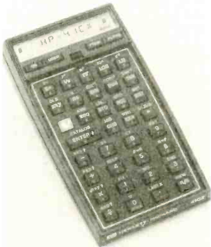
FIG. 15—THE HP-41 IS A combination handheld calculator and controller for the HP-IL.
