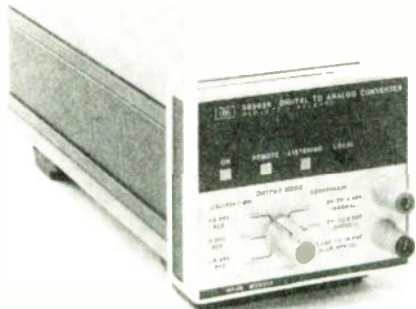
FIG. 8—THE HP 59303A digital-to-analog converter accepts a string of serial ASCII characters, then converts any three consecutive input digits to an analog output voltage.
