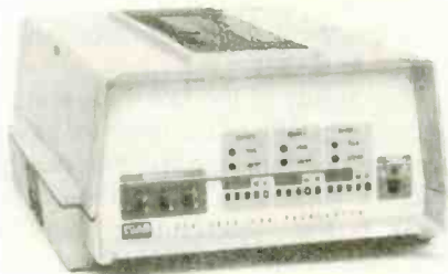
FIG. 14—THE FLUKE 1120A IEEE-488 translator can up-grade an instrument not specifically designed for the GPIB.
