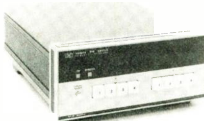
FIG. 10—THE HP 59307A DUAL VHF switch module provides two 1P4T switches controllable by the GPIB.
