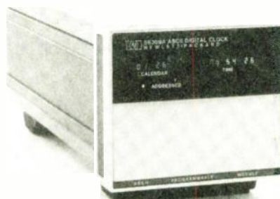
FIG. 11—THE HP 59309A GPIB digital clock displays month, day, hour, minute, and second, and upon command will output time via the interface bus.
