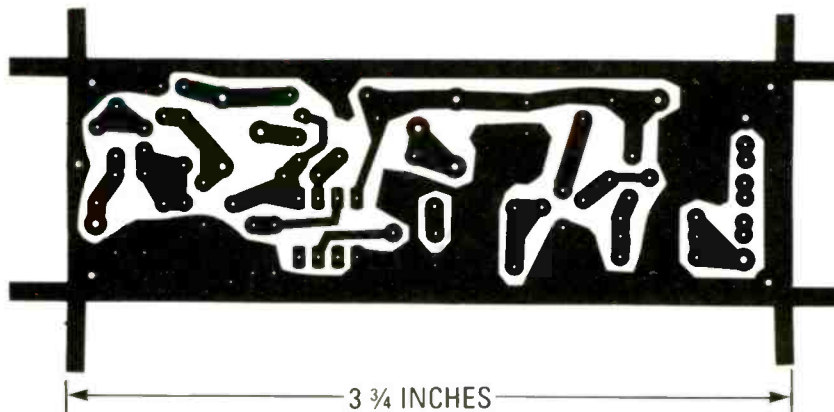
THE INFRARED TRANSMITTER board shown here is full sized.
