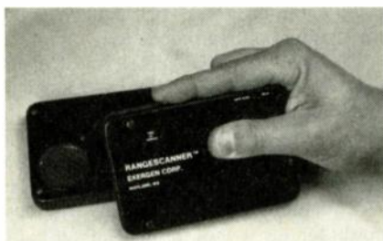
FIG. 13—THE ULTRASONIC RANGESCANNER measures distance and uses a Polapulse battery for power.
