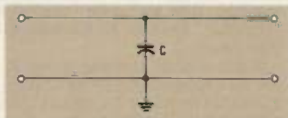
FIG. 4—A SINGLE CAPACITOR, installed as shown, can be used to filter out differential-mode interference. To handle common-mode interference, the capacitor should be installed between each line and ground.
