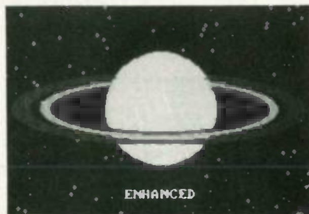
FIG. 5b—BUT WHEN PROCESSED by a Video Enhancer an RGB color signal can look quite good on a monochrome monitor because the device converts each color to an individual shade of grey.
