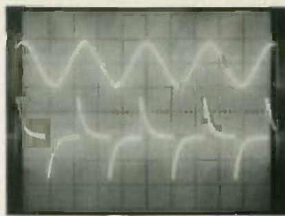
THE UPPER TRACE is a 3-kHz input signal from a signal generator. The bottom one is the output that results.
