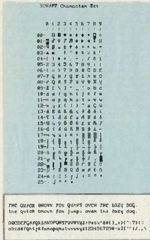
FIG. 2b—SINCE DIGICON GENERATES the characters independently through dot-addressable graphics, it can generate various type faces, such as this "script" font.
