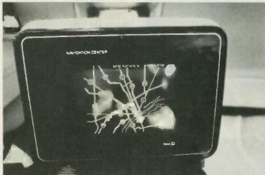
FIG. 4—THE NAVIGATION SYSTEM in the Questor can display area, region, or state maps on one of the vehicle's center-console CRT's.
