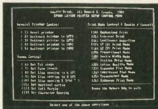
FIG. 1—PRINTER CONFIGURATION SOFTWARE lets the user program a printer's function(s) through menu selection instead of a BASIC program. This menu, from Adapta-Print, allows direct selection of forms control and printer ports. However, while the user can select a serial port for the printer, the port had to be previously configured for serial parameters through the OOS MOOE command.
