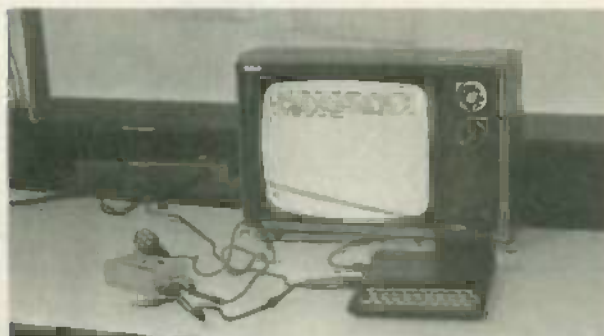
FIG. 2—THE COMPUTER with audio amplifier and mike connected to cassette interfaces. The program seen on the screen is a representation of the machine code program.
