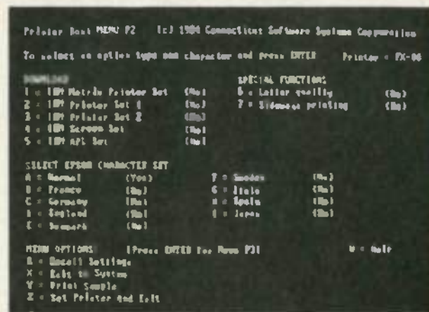
FIG. 3—THE PRINTER BOSS can actually configure a printer so the printer itself "thinks" it's IBM compatible. It does this by downloading a character set(s) into the printer's memory. The only limitation to this method is that it is presently available only for the Epson FX printer series.
