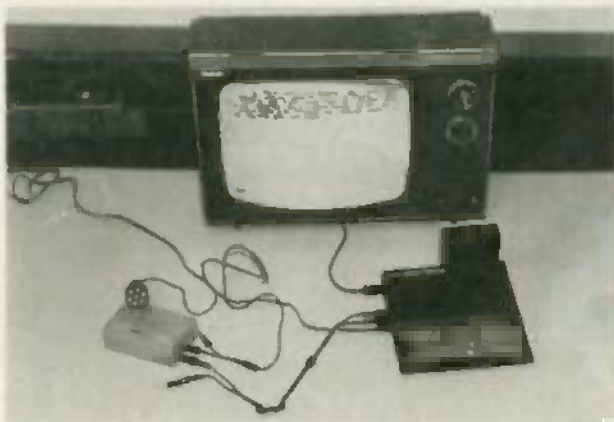
FIG. 3—MICROPHONE IS CONNECTED TO AMPLIFIER which enters the ear-jack of the computer. Mic-jack is unconnected but will connect to another amplifier and speaker.
