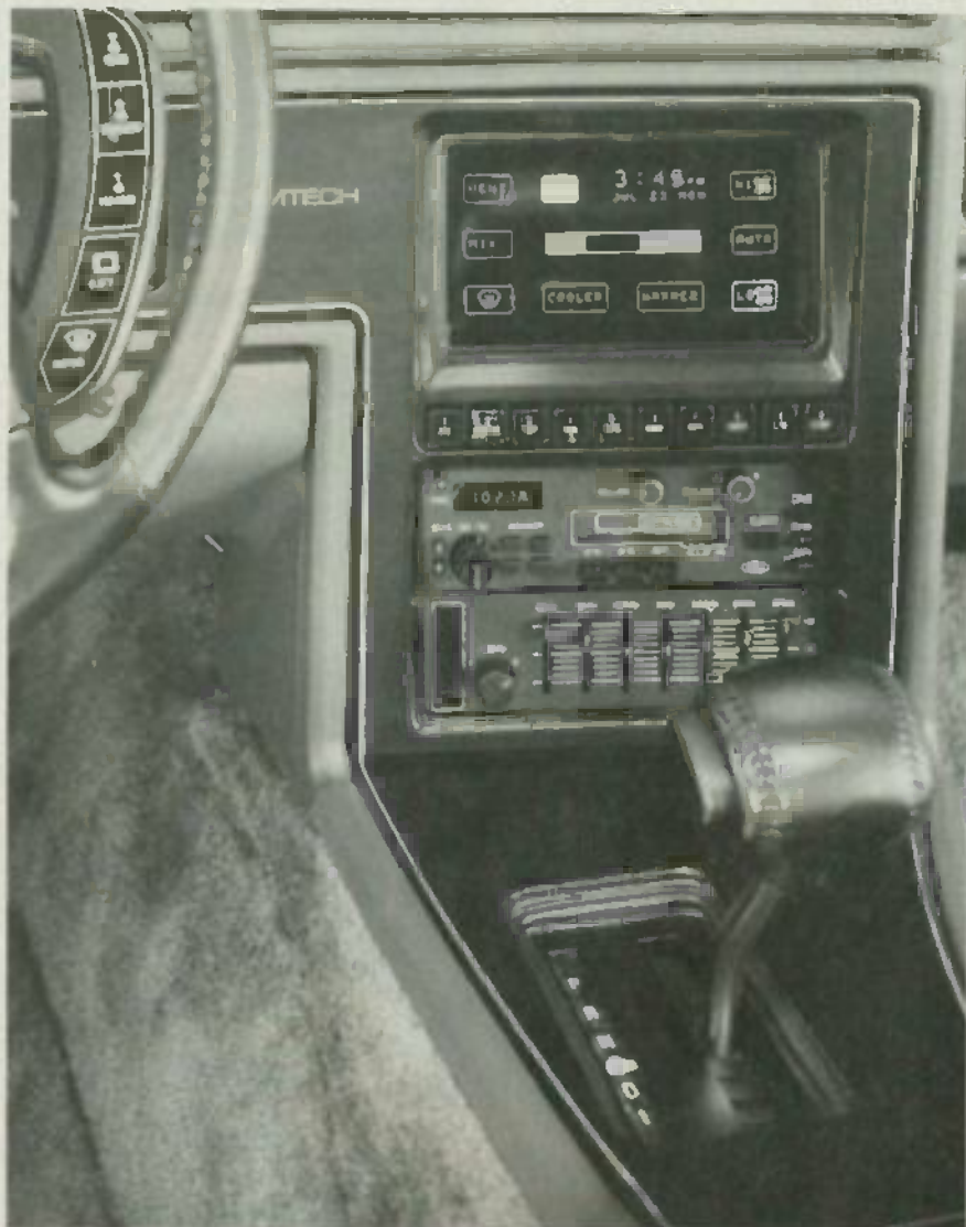
FIG. 1—A CRT WITH TOUCH-SENSITIVE SCREEN is used to replace traditional mechanical climate controls in this Mark VII Comtech, a limited-production vehicle from Ford.
