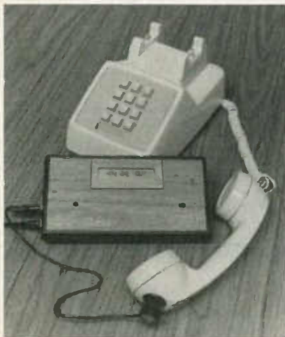
PHONE READER FOR THE DEAF. The compact, battery-powered device attaches to any phone.
