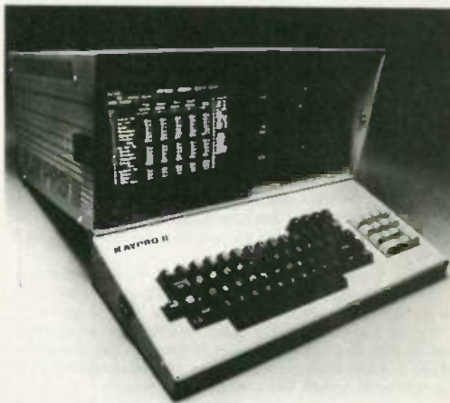
FIG. 3—THE KAYPRO II shown here, can read several different disk formats.
