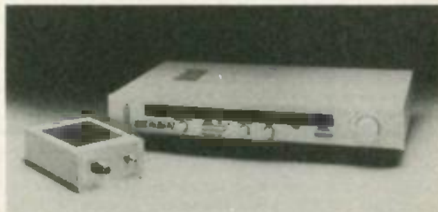
FIG. 1—SATELLITE TV RECEIVER. Features of this unit (KLM Sky Eye V11X) include variable speed scanning for fast scanning of the satellites or frame-by-frame viewing of each of the 24 transponders of a satellite. Note that this receiver uses an external downconverter, shown beside it.
