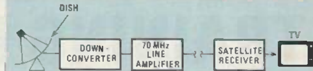
FIG 6—IF SIGNAL STRENGTH is inadequate, or if more than one satellite receiver is to be used, a line amplifier can be placed between the downconverter and the receiver.
