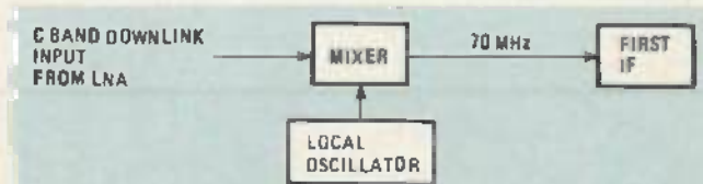
FIG. 5—IN A DOWNCONVERTER, the downlink signal is mixed with the output of a local oscillator to produce a 70-MHz IF.
