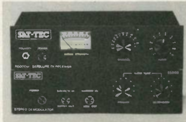
TWO-CHANNEL SOUND. Some receivers can have stereo capability added to them through the addition of an external stereo demodulator.
