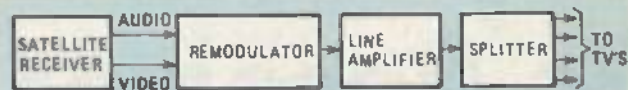
FIG. 8—IF A NUMBER OF TV SETS are to be connected to the remodulator, or remodulator-equipped satellite receiver, a line amplifier may be required. The line amplifier connects to a signal splitter whose output feeds the antenna input terminals of the TV sets.
